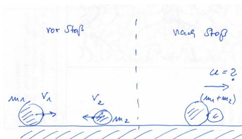
$$\begin{aligned} \underbrace{m_1 v_1 + m_2 v_2}_{=p_{ges,vor}} &= \underbrace{(m_1 + m_2)u}_{=p_{ges,nach}} \\ u &= \frac{m_1 v_1 + m_2 v_2}{m_1 + m_2} \\ u &= \frac{m_1}{m_1 + m_2} v_1 + \frac{m_2}{m_1 + m_2} v_2 \end{aligned}$$
